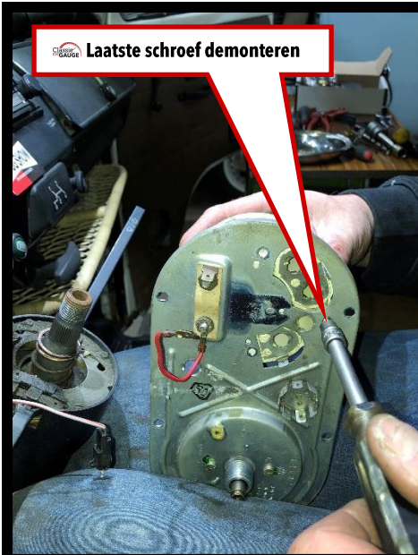
Plastic behuizing demonteren
