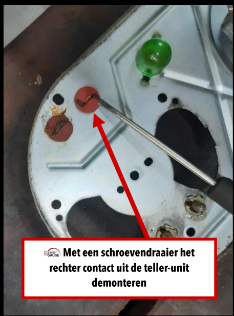
Remove feed-through contact from the backplate
