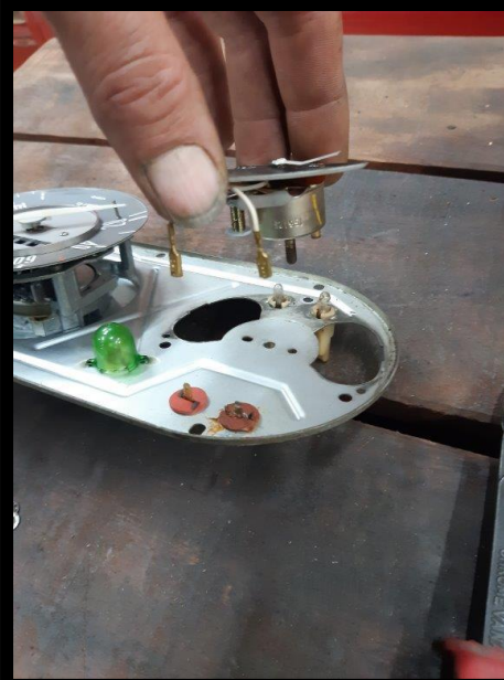
Now Gently!!!! Remove the screen of the original fuel gauge with a small screwdriver
