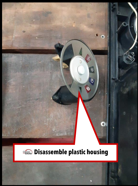
Remove the FINAL screw of the original fuel gauge with and remove the gauge
