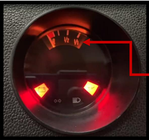
The dial of the Classic Evo Gauge will be orange the entire reserve
