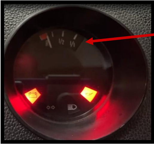
If the meter runs out of reserve, the dial of the Classic Evo Gauge will no longer give a LED indication
